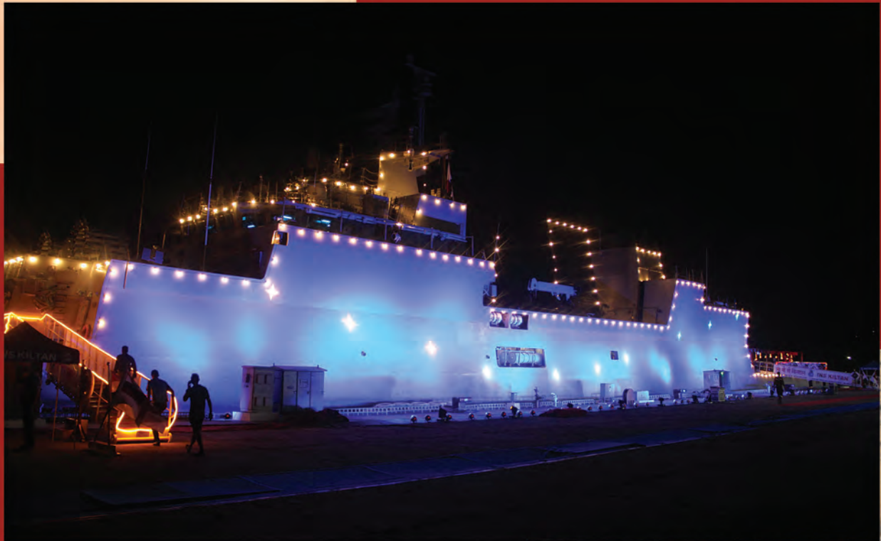
The Superstructure of INS Kiltan (3 rd Anti Submarine Warfare Corvette) has been made of Carbon Fibre Composite Material and is Integrated with the Steel Hull of the Ship. GRSE is the First Shipyard in the Country to have achieved this feat. This feature of INS Kiltan has reduced the Overall Weight of the Ship
