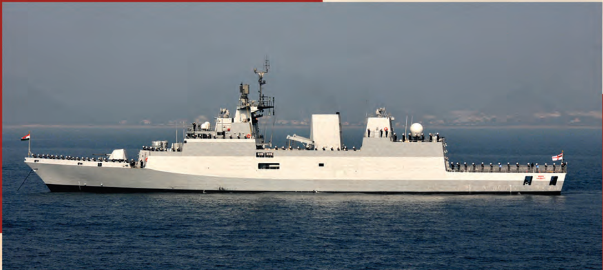
The Superstructure of INS Kiltan (3 rd Anti Submarine Warfare Corvette) has been made of Carbon Fibre Composite Material and is Integrated with the Steel Hull of the Ship. GRSE is the First Shipyard in the Country to have achieved this feat. This feature of INS Kiltan has reduced the Overall Weight of the Ship
