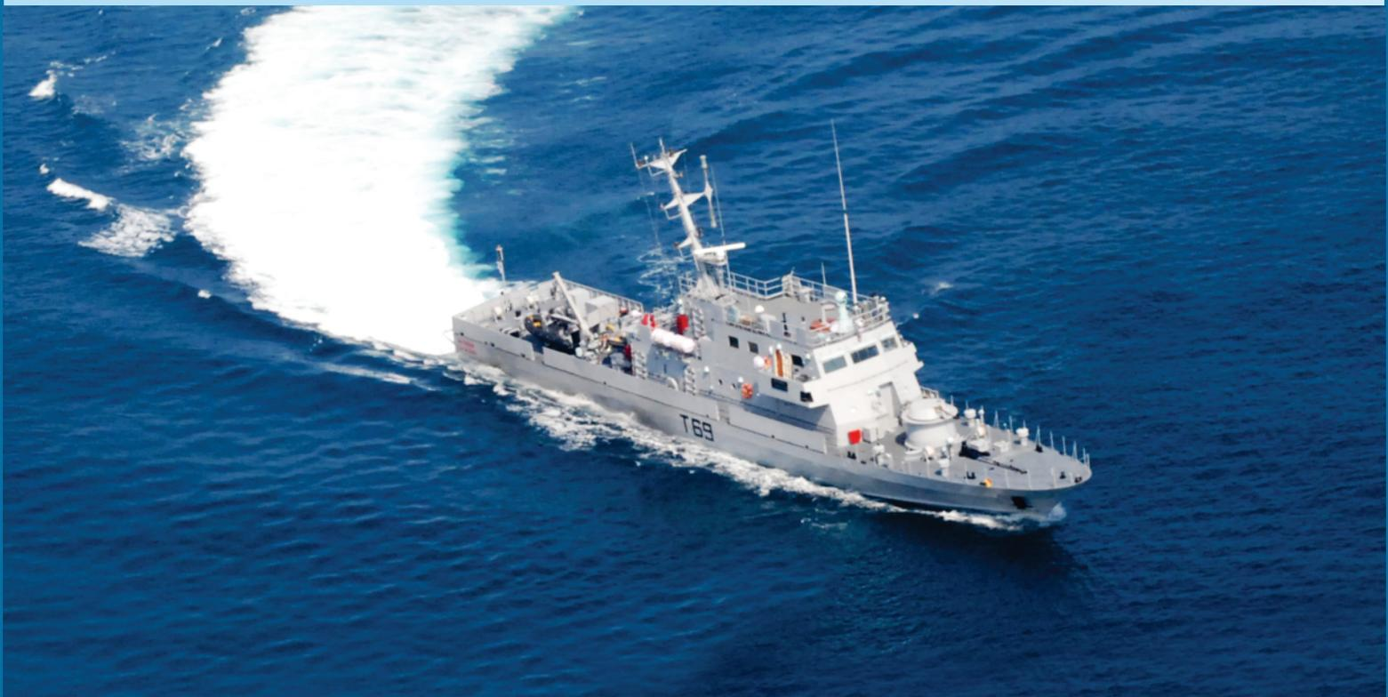
Water Jet Fast Attack Crafts promise to transform naval shoreline operations by packing a powerhouse punch of agility and speed. These WJFACs are ideally suited for interception of fast moving surface craft and will duly perform Anti-Smuggling, Fishery Protection and Search & Rescue Operations. The ships are fitted with Hamilton Water Jets.
